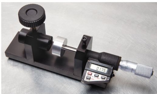
Calibration fixture 2U-16U sensors English/Metric 855578-001
